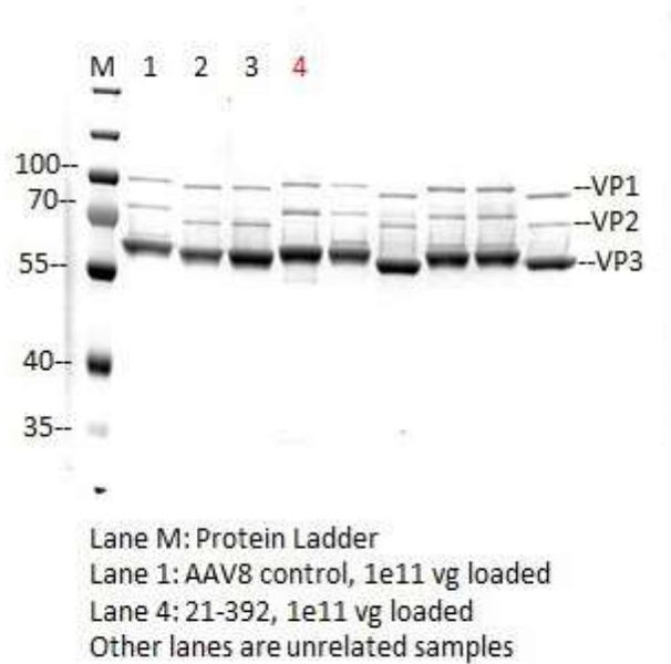
Fig. 1. SDS-PAGE and InstantBlue Staining of purified AAV8-empty (Lot: 21-392)
